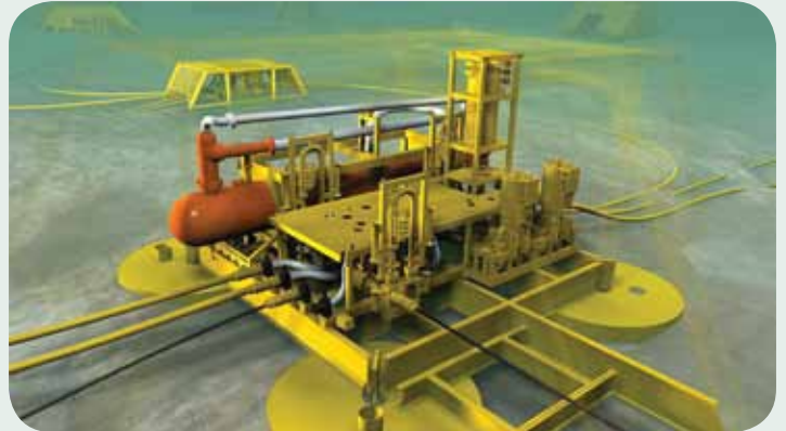
TORDIS - The world's first full field subsea separations system
